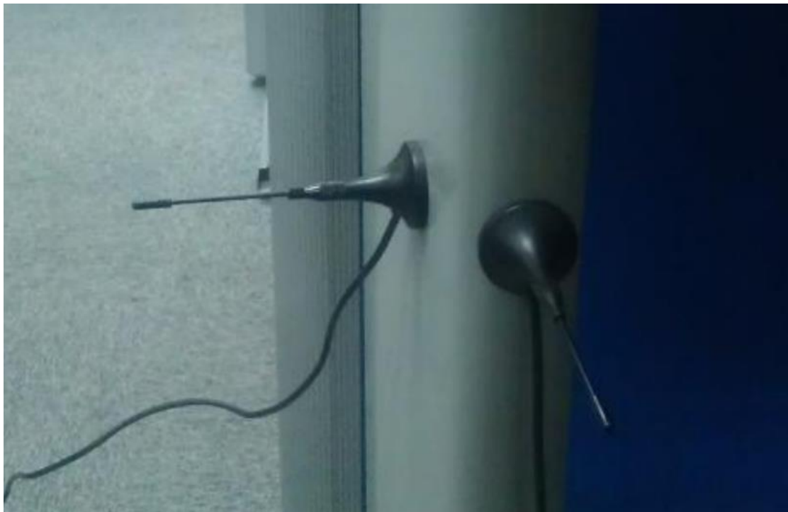
Figure 6.3 Isolation by antenna orthogonal polarization
