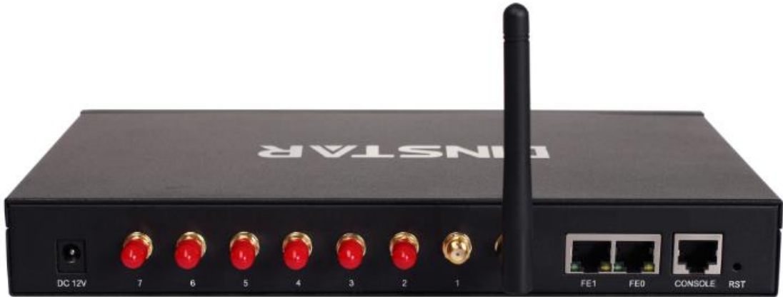
Figure 1-3-2 Rear view of DWG2000E-8G/8C
