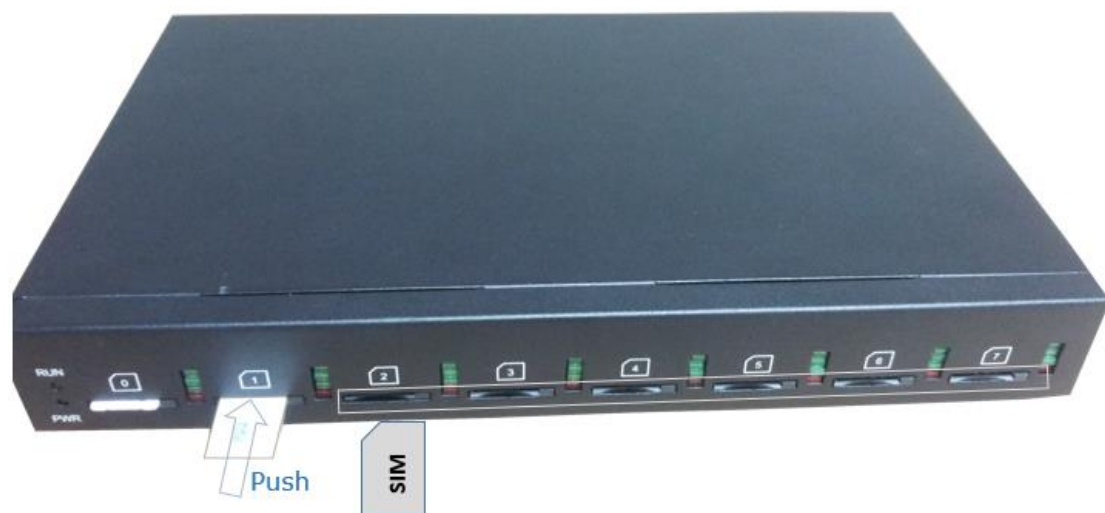
Figure 2-2-1 SIM Card installation
